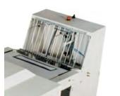
This simple stacker aloow to collect collar and cuffs after fusing, this system will be perfect also without cooling system because the parts will have their time to cool on the stacker skid.
