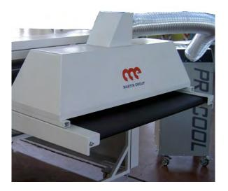
Active cooling system is a powerful active cooling fridge group separate from fusing machine, with this system you can also regulate the cooling temperature.
